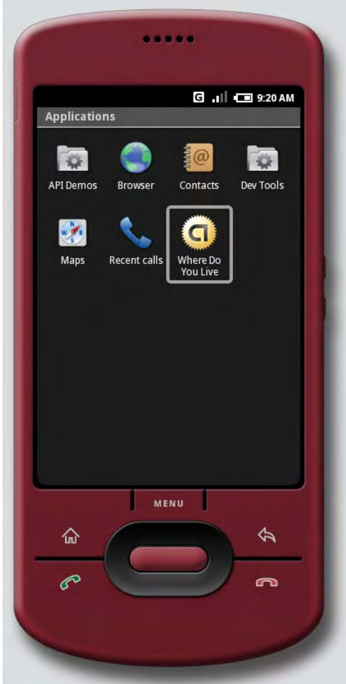
Figure 1.7 Applications are listed in the launcher based on their Intent Filter. In this example, the application titled “Where Do You Live” is available in the LAUNCHER category.
