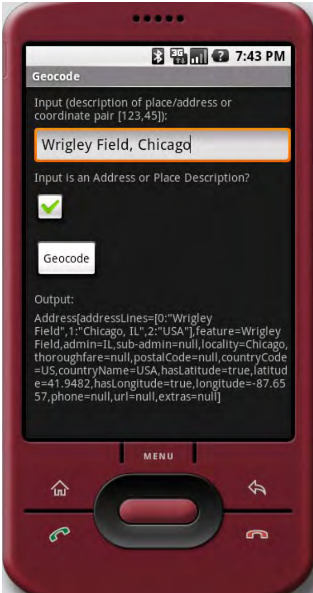
Figure 11.7 A Geocoder usage example that demonstrates turning an address String into an Address object which provides latitude and longitude coordinates.
