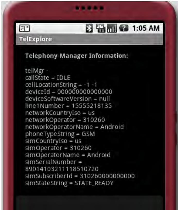
Figure 7.2 Displaying device and phone network meta information obtained from the TelephonyManager class.
